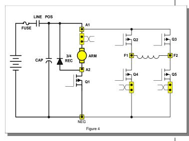
By energizing the transistors in pairs, current can be made to flow in either direction in the field. The field and armature control circuits typically operate at 15KHZ, a frequency range normally above human hearing. This high frequency, coupled with the elimination of directional contactors, provides for very quiet vehicle operation.
